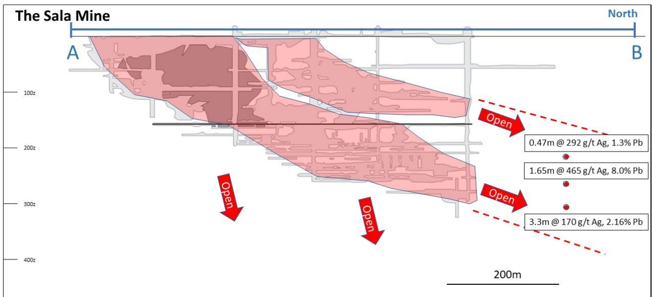
Figure 3: Long section of the Sala Silver mine looking west.
